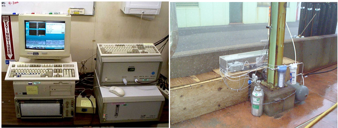
Figure 27. Fiber-coupled spectroscopy instrumentation (left) located in the control room. Multi-pass cell and auto-calibration hardware (right) housed in boxes outside.
