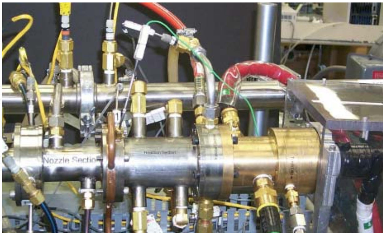
Figure 3-4. Photograph of torch, injector, reactor and nozzle assembly, flow is right to left.
