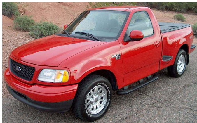
Figure 13. The 16-Valve, 5.4 liter Ford F-150 ICE vehicle that operates on 100% hydrogen.
