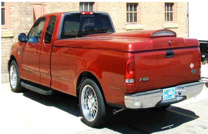
Figure 14. 32-Valve, 5.4 liter Ford F-150 converted to operate on 100% hydrogen by ETEC.
