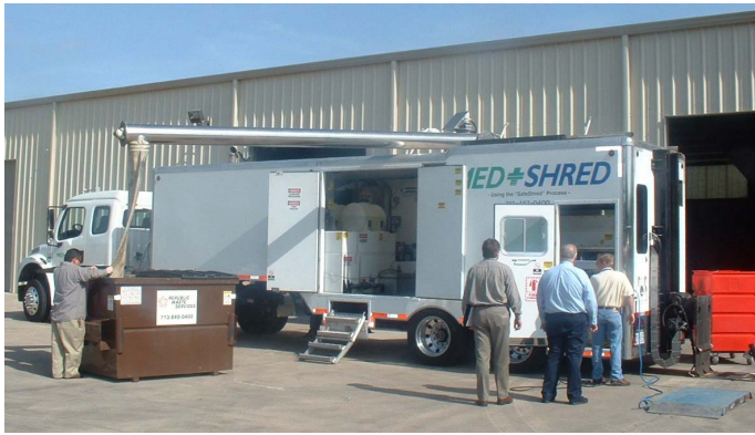
Figure 2. Typical truck-mounted Med-Shred medical waste treatment system seen during a treatment capability demonstration.
