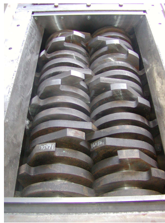
Figure 5. A top view looking inside a low-speed, high torque shredder. Teeth on counter-rotating discs bite into and pull material between the two shafts, cutting the material into smaller pieces.
