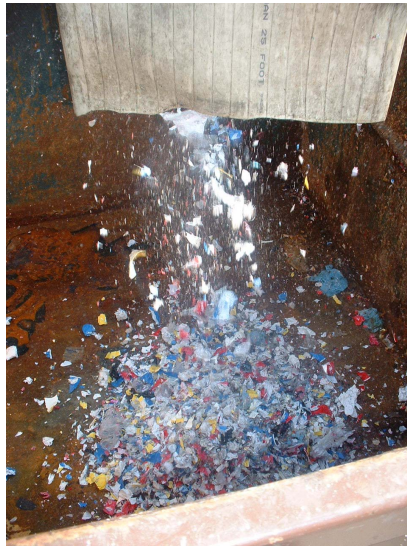
Figure 7. Typical appearance of shredded and disinfected medical waste. This photo shows shredded and treated surrogate medical waste materials, consisting of non-contaminated paper materials, plastic materials (plastic drinking cups), cloth materials (shop rags), and glass materials (glass drinking cups).
