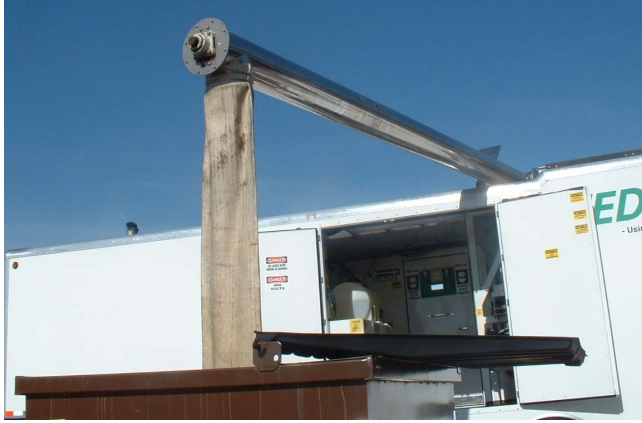
Figure 6. The boom is used to transport treated waste from the processor to a hospital compactor or other container for the treated waste.
