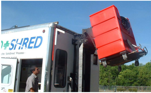
Figure 4. A plastic cart containing surrogate medical waste is lifted and dumped into the shredder hopper during a treatment capability demonstration.
