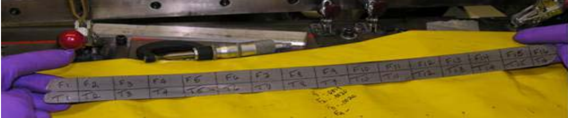
Figure 3. Graded U-Mo foil. DU-10Mo foil produced by hot rolling.
