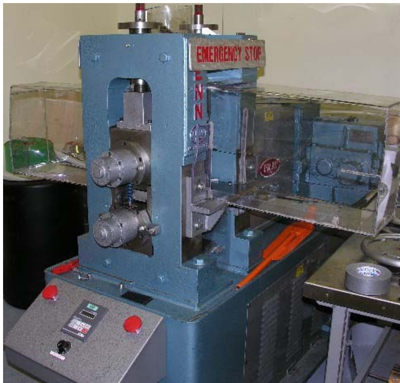
Figure 10. Foil rolling mill. The containment box is shown on either side of the rolling mill.
