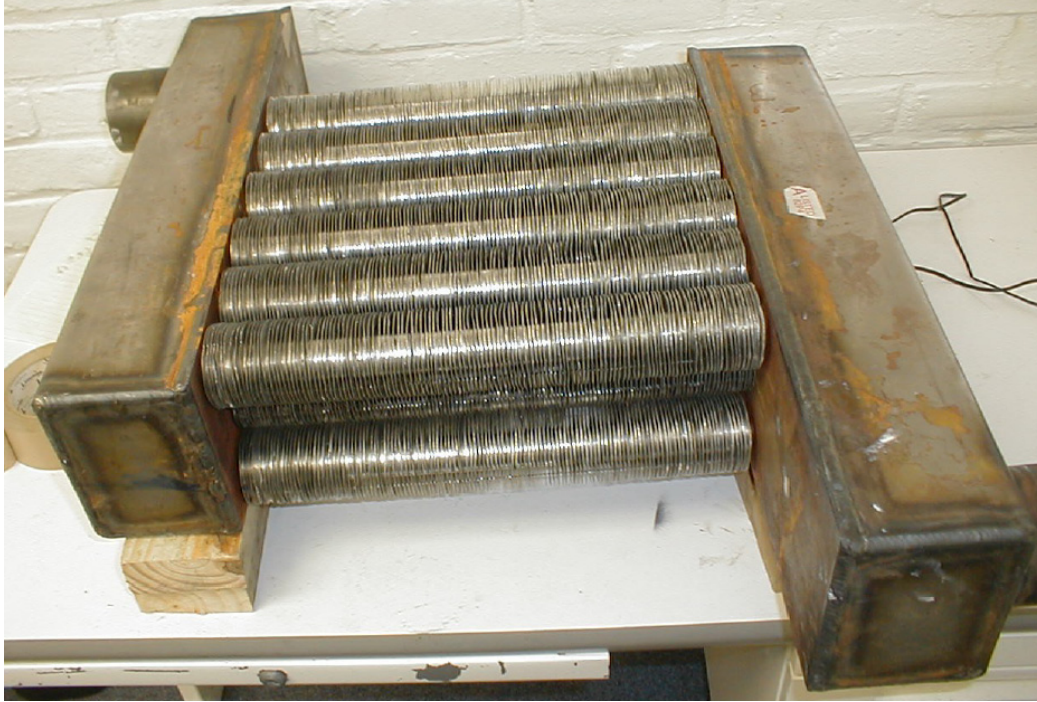
Figure 7-3. Photograph of the test apparatus with enhanced finned tubes and inlet and outlet plena.
