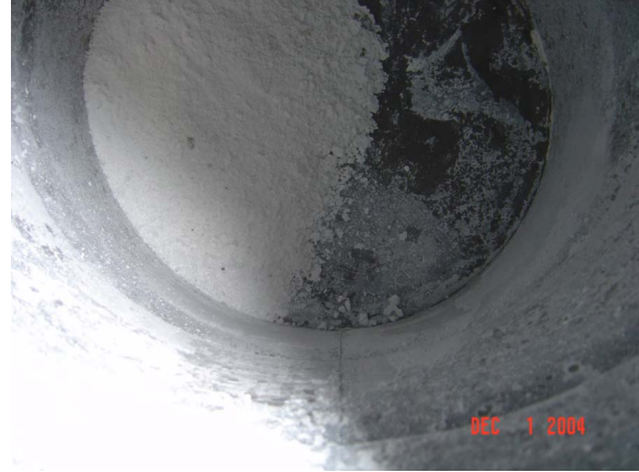
Figure 15. ANL#1174 after treatment with humidified carbon dioxide.
