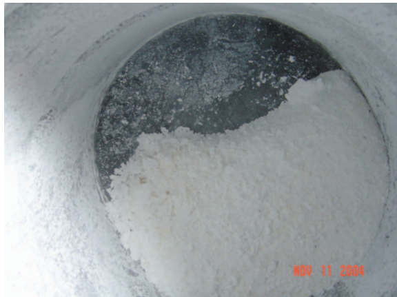
Figure 8. ANL#630 after treatment with humidified CO 2
