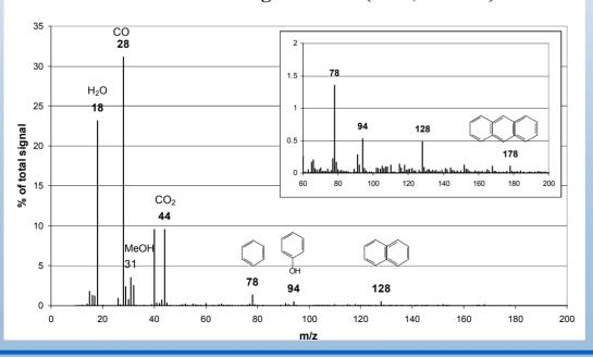
Under oxidative cracking conditions, H<sub>2</sub> (not shown), water, CO, and CO<sub>2</sub> predominate. Hence the role of the catalyst to be added is to finish the conversion and catalyze the water-gas shift.
