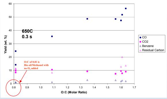
Gas-phase partial oxidation leads to high CO yields with low CO<sub>2</sub>.
