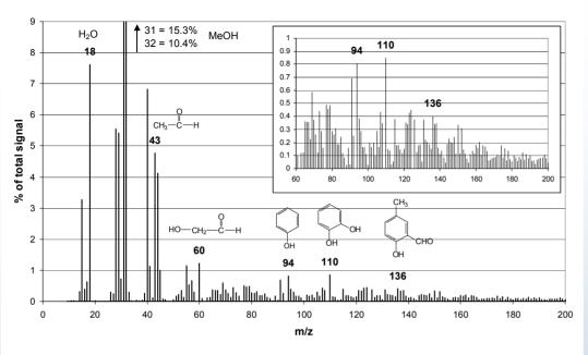
Under thermal cracking conditions, unconverted methanol and secondary products from the bio-oil predominate.
