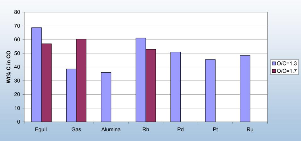
By-products are typically above equilibrium levels and thought to be generated from non-volatile species in aerosols and processes in the gas phase.
