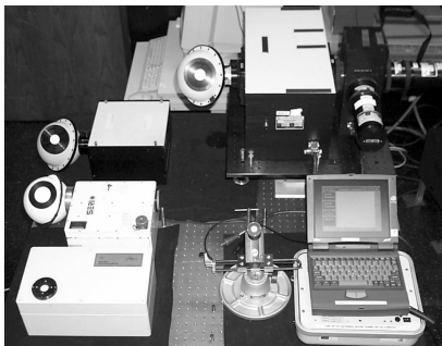
Figure 1. NREL spectroradiometers. Clockwise from front left: Li-1800 [0.3-1.1 \mu\text{m} ], Geophysical Environmental Research (GER) [0.35 -2.4 \mu\text{m} ], Optronic Laboratories (OL) OL-754 [0.18-0.8 \mu\text{m} ], OL-750 [0.25 -2.4 \mu\text{m} ], Analytical Spectral Devices (ASD) FieldSpec FR [0.35 -2.4 \mu\text{m} ]
