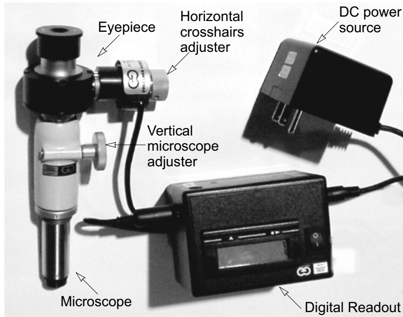
Figure 4.4. Components of the digital filar microscope used for measuring sorption-induced strain in coal.
