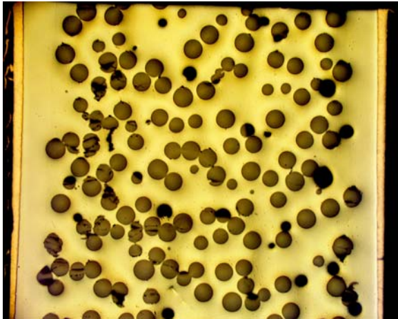
Figure 17. Photograph of 0.4" diameter Zr matrix dispersion "fuel" extrusion longitudinal cross section. Spheres measure approximately 0.5mm in diameter.
