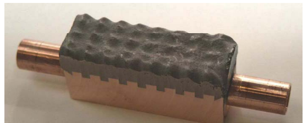
FIG. 2. Sample with 3-mm cubic projections machined into the Cu alloy substrate and plasma sprayed with 10 mm of beryllium.
