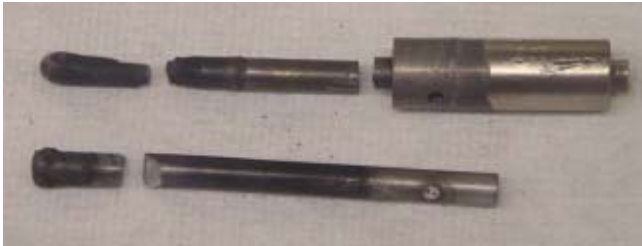
FIG. 1. Beryllium rods immersed in molten Flibe at 530°C for 150 hours demonstrated the effect of galvanic coupling in accelerating beryllium dissolution. The top rod was electrically coupled to the nickel crucible while the bottom rod was insulated from it.
