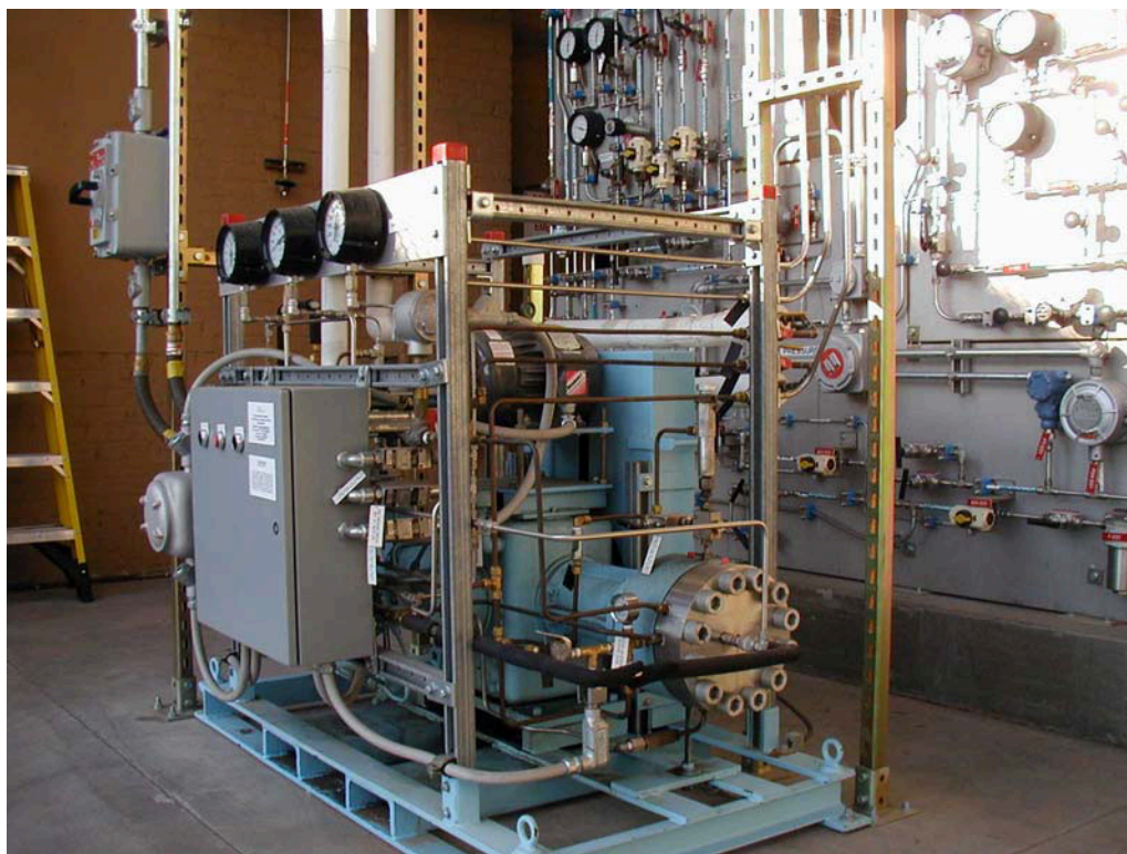
Figure 2.4. Pdc Machines, Inc. diaphragm hydrogen compressor.
