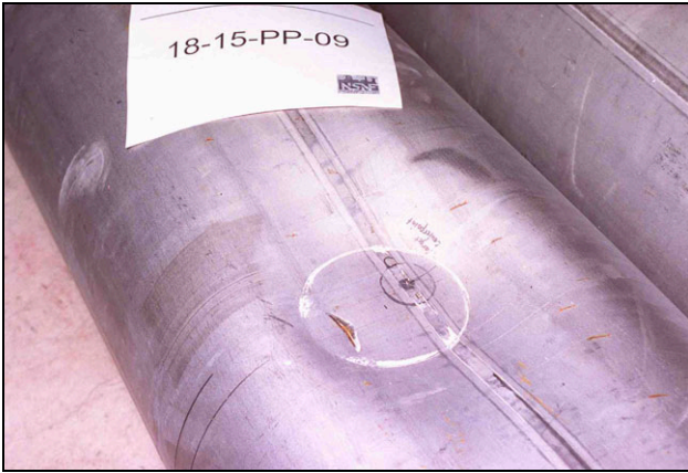
Figure 13. Deformed Body of Canister 09
