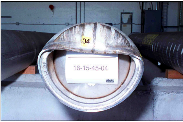
Figure 7. Deformed End of Canister 04
