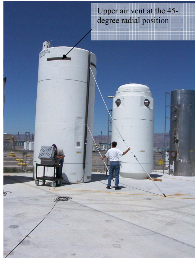
Fig. 3. Thermocouple measurements were taken using a thermocouple ladder.
