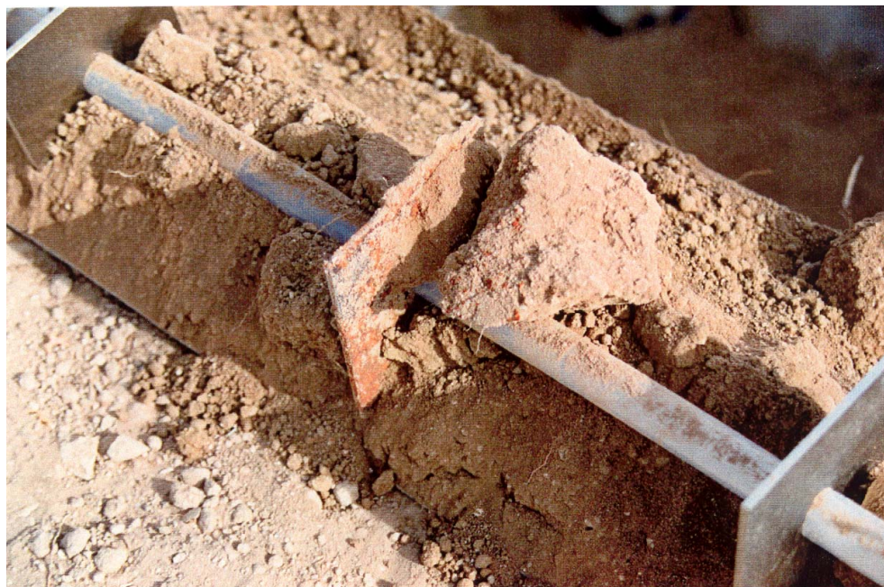
Figure 3-4. Corrosion test coupons removed for analysis after 3 years of burial near the Radioactive Waste Management Complex (photo reproduced from Adler-Flitton et al. 2001).
