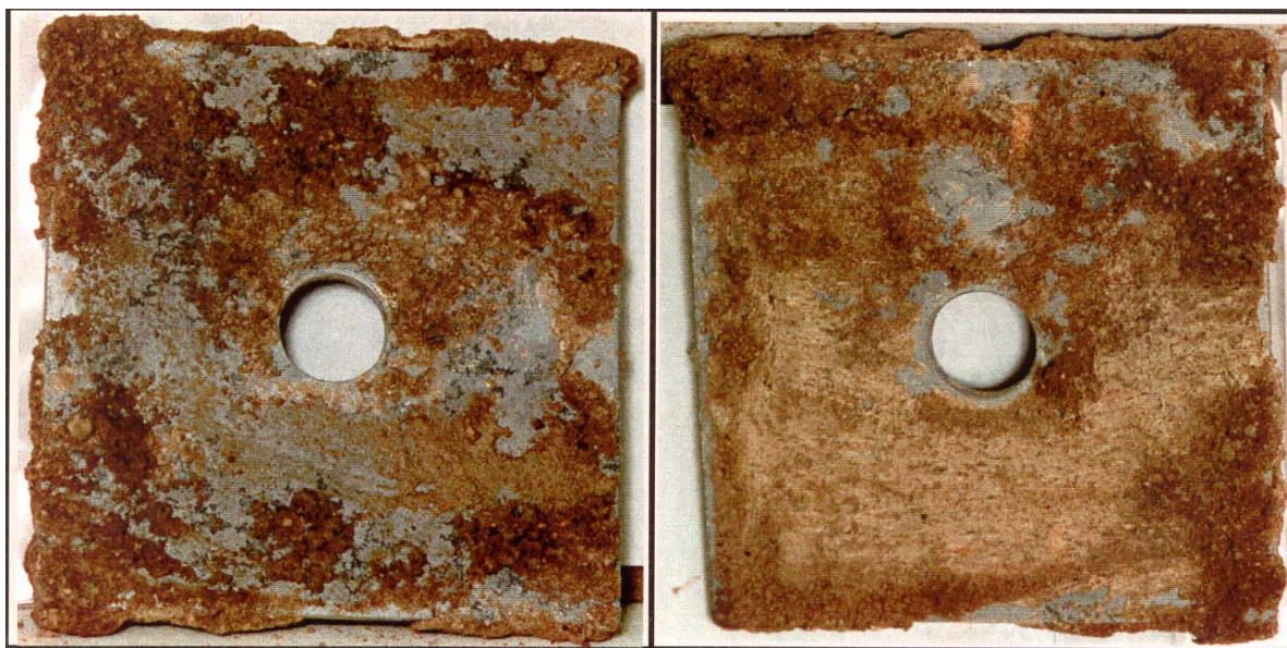
Figure 3-5. Beryllium coupon (front and back) recovered after 3 years of burial, before cleaning (photo reproduced from Adler-Flitton et al. 2001).
