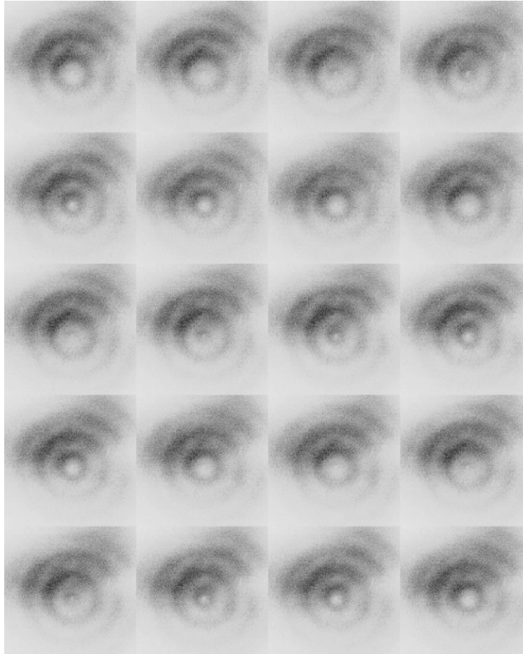
Figure 5. Time-lapse picture of successive frames of the traveling wave images showing the emergence of the wavefront from the center of the plate.
