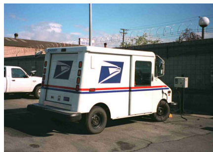
Figure 16. U.S. Postal Service light-duty electric delivery vehicle being charged at Southern California Edison.
