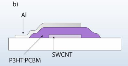
SWCNT Deposition by spraying of nanotube dispersion in ethanol onto heated (65°C) substrates
