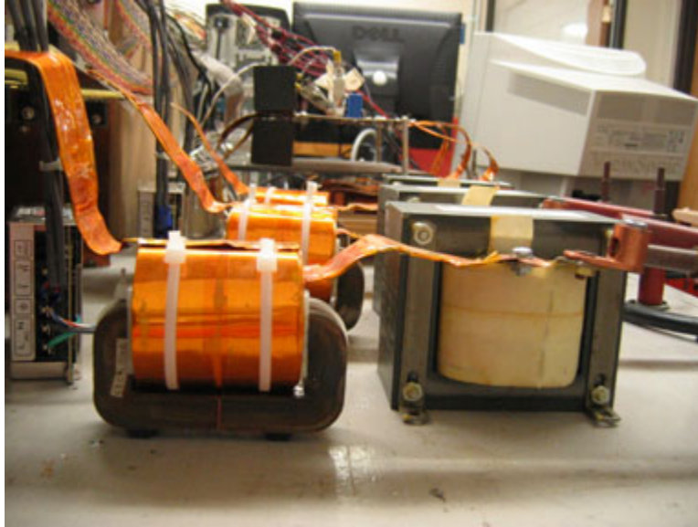
Figure 6.6: Filter inductors at one converter terminal
