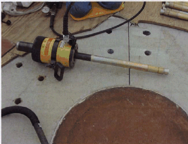
Drillco Flush Mount Anchor inserted in hydraulic setting tooling.
