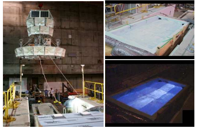
FIG. 2: (color online) Left: The ANITA payload (center) above and downstream of the ice target (here covered). Right top, target with cover removed, in ambient light. Right bottom: ice target illuminated from interior scattered optical Cherenkov radiation.
