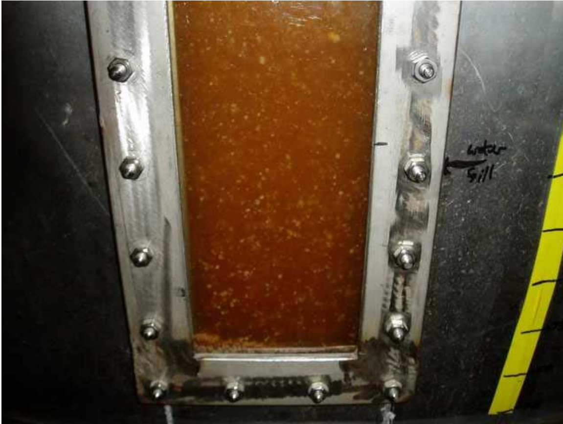
Figure 3.1.14 Photo showing typical yeast pellets. Pellet diameters ranged from 0.5 to 10 mm.
