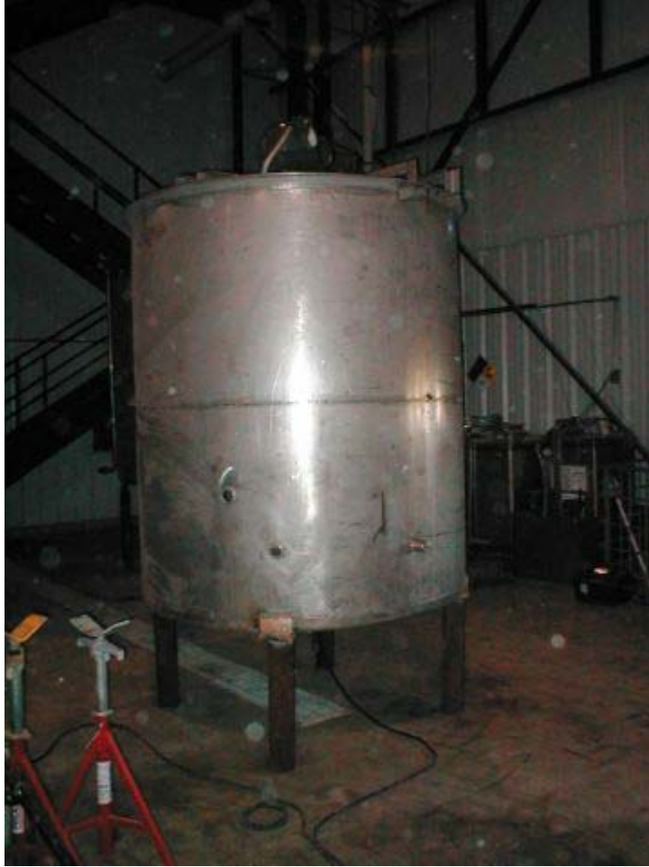
Figure 3.1.2 Tank T-201- 1, 250 Liter (8' by 6' diameter- under construction)
