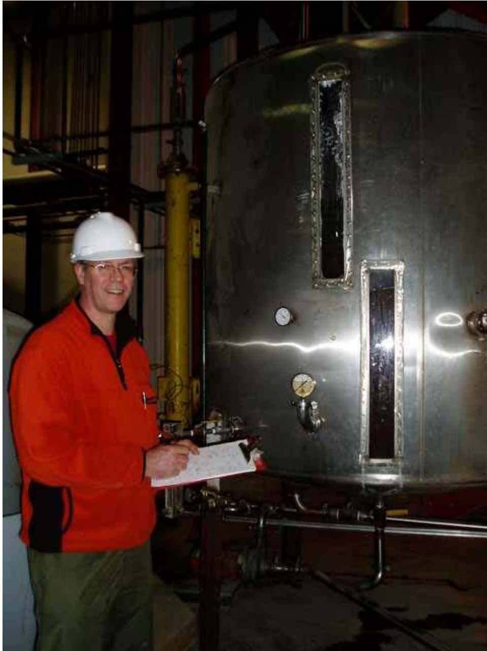
Figure 3.1.9. Dr. Dale at shake-down trial of 3/19. Cooling external Heat Exchanger HX 301(in yellow paint) is on the left, circulating pump P-301 can be seen below HS/LE Reactor T-301.
