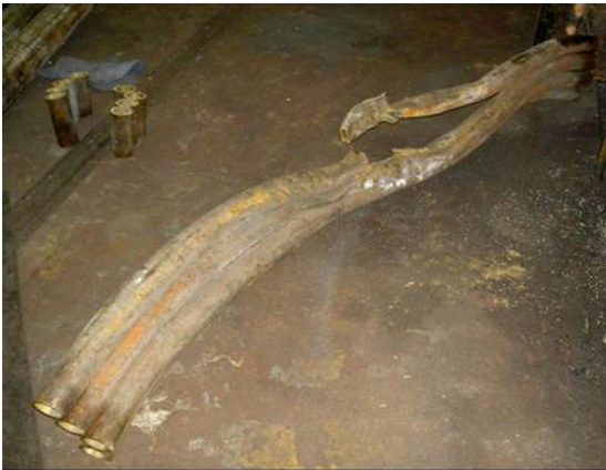
Figure 20. Skirt Damage, Collision with BOF Vessel.
