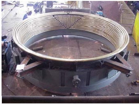
Figure 18. Al-Bronze Skirt before Installation
