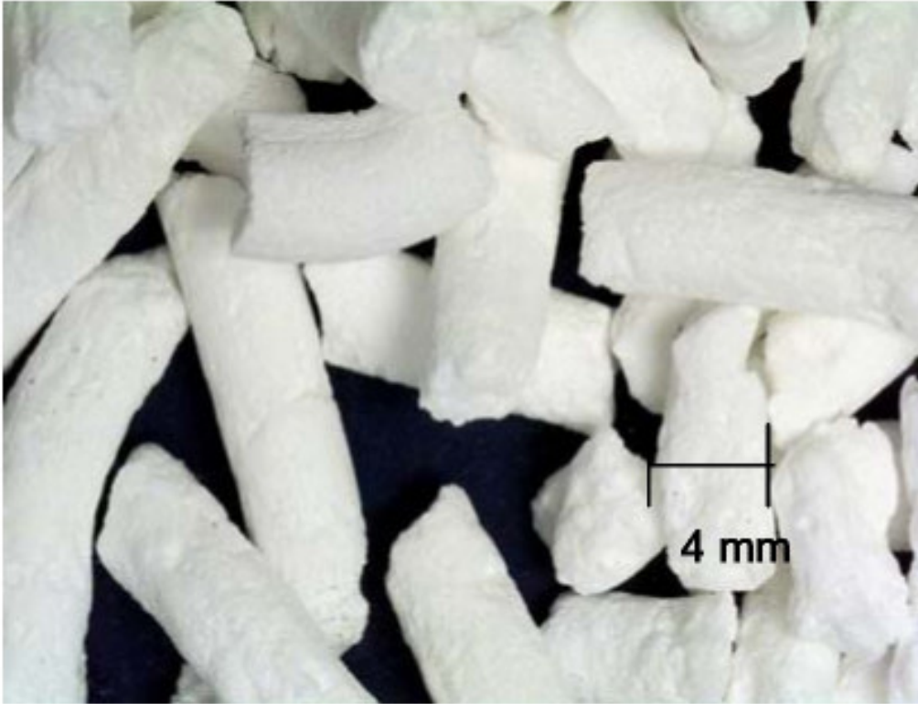
Figure 4: Photograph of SBA micro-porous filter media. Nominal diameter of the media is 4 mm.
