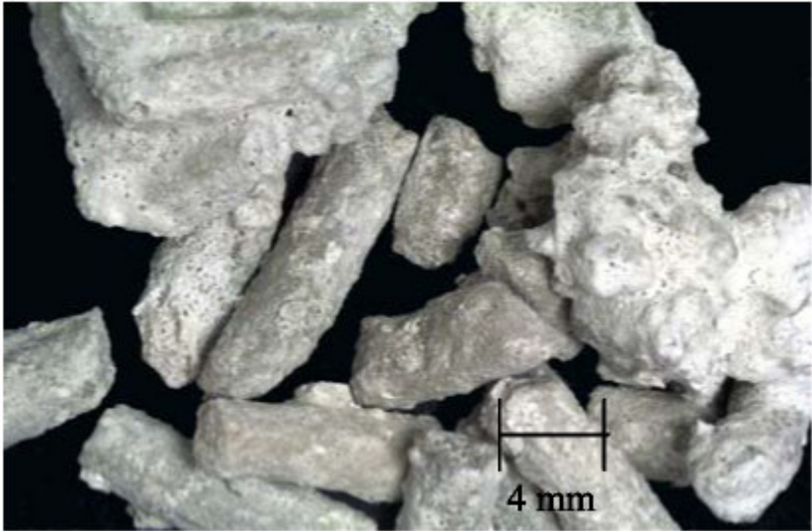
Figure 10: SBA micro-porous filter media after removal from bed filter.
