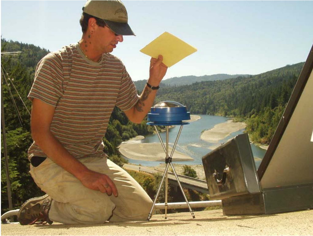
Figure 5. Energy Technician Stephen Kullmann evaluates shading on a solar-equipped rooftop overlooking the Klamath River
