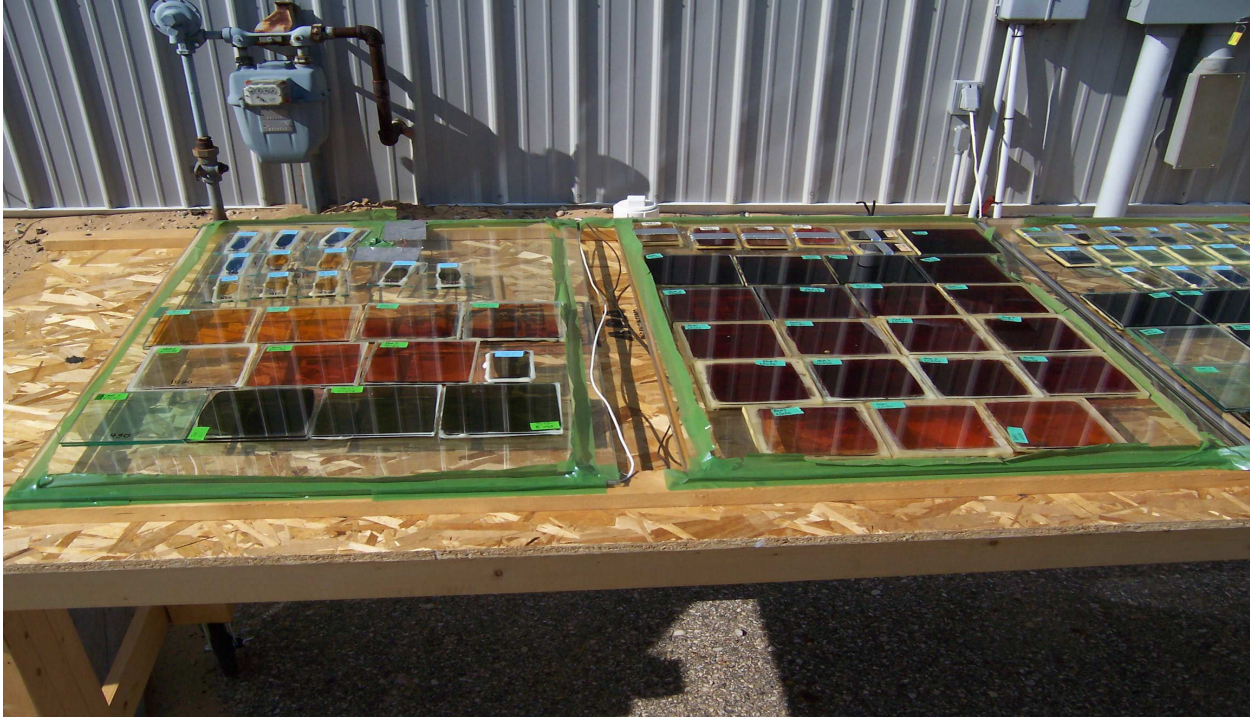
Picture above is parts being test in sunlight and heated to 85 °C
