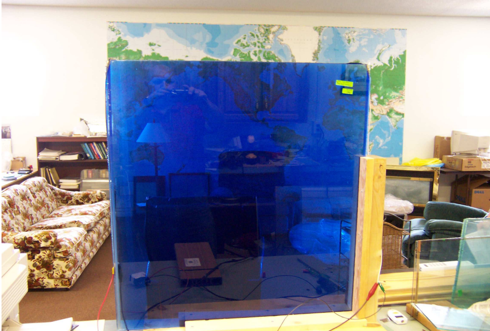
Picture above is an SRT laminate with a blue film at 75 °C
