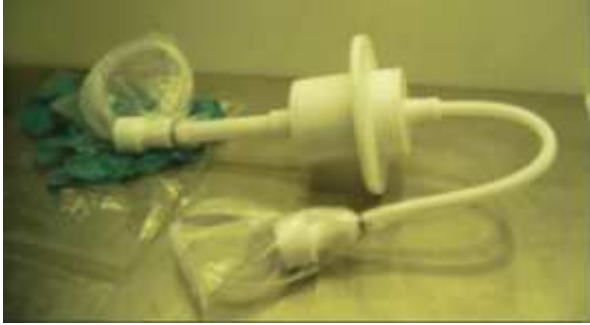
Fig. 5. Photograph of a finished chamber of the type illustrated in fig. 1. The two pipes are used for xenon recirculation and as conduits guiding the detector wiring to the outside. Electrical feedthroughs are, in this prototype, conventional (metal-ceramics), mounted after the fluoropolymer-to-metal transition. The high potential ( \sim 5 kV) required for the cathode is fed through the pipe opposite to the one feeding the anode, grids and APD potentials and signals.
