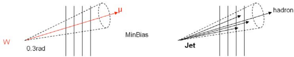
Figure 52 Schematic of an isolation cut: the number of particles in a given layer that are within a cone are counted and if the number found is less than some value the particle is considered to be “isolated” and if it is larger than that value it is not isolated. Left cone illustrates a muon from a W event and the right cone illustrates a hadron associated with a jet of particles.
