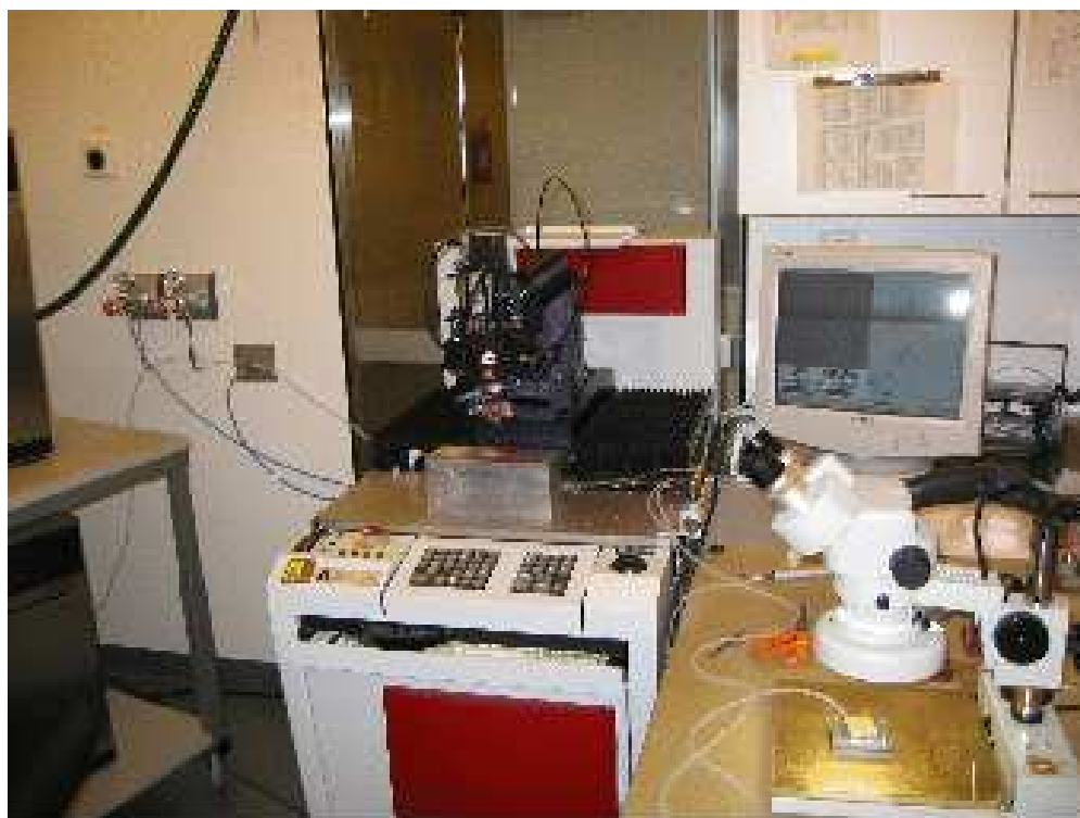
Figure F.15: Automatic wire-bonding machine in clean room facility at Helsinki Institute of Physics.
