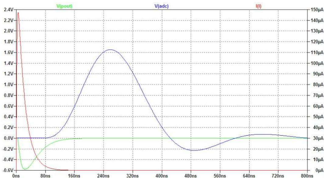
Figure E.5: Transient analysis, R_{cr} = 35 \text{ Ohm} .
