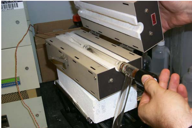
Figure 4. Glove oven with thin-film Ag deposited substrates and Tellurium in vacuum-sealed quartz vessel
