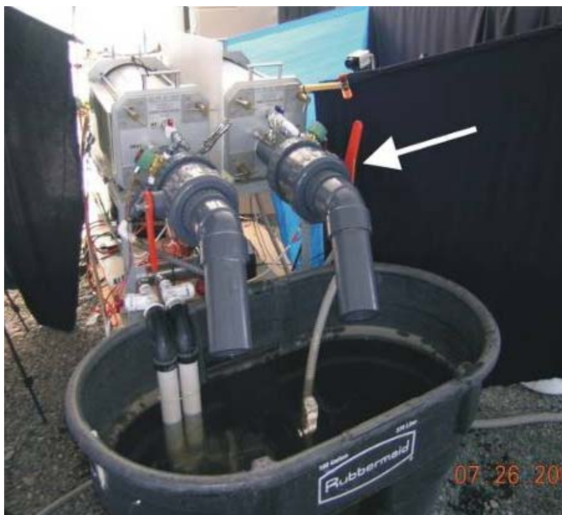
Figure 2.8. PVC Drain Valves (10.2 cm; orange handles illustrated by white arrow) Mounted on the End of the Hyperbaric Chambers
