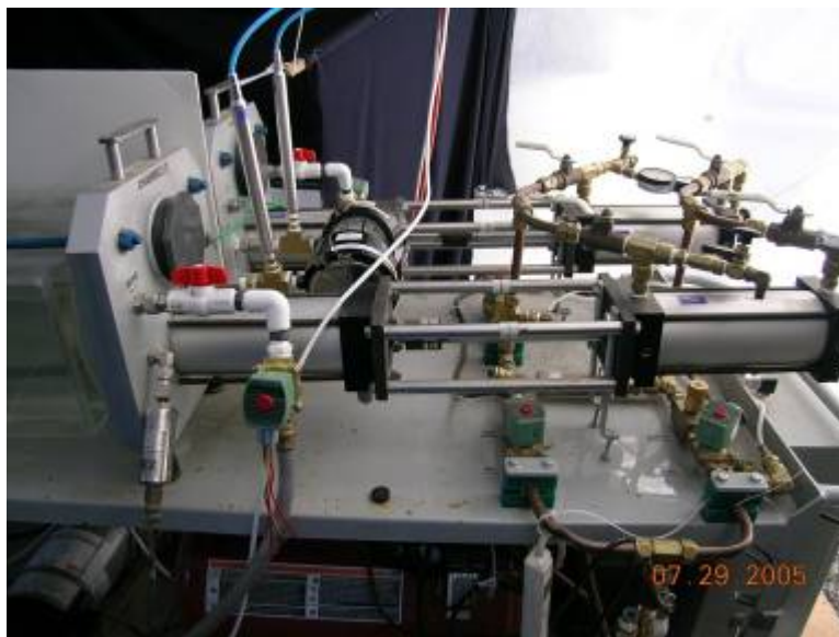
Figure 2.6. Hydraulic Cylinders Connected to Pneumatic Cylinders
