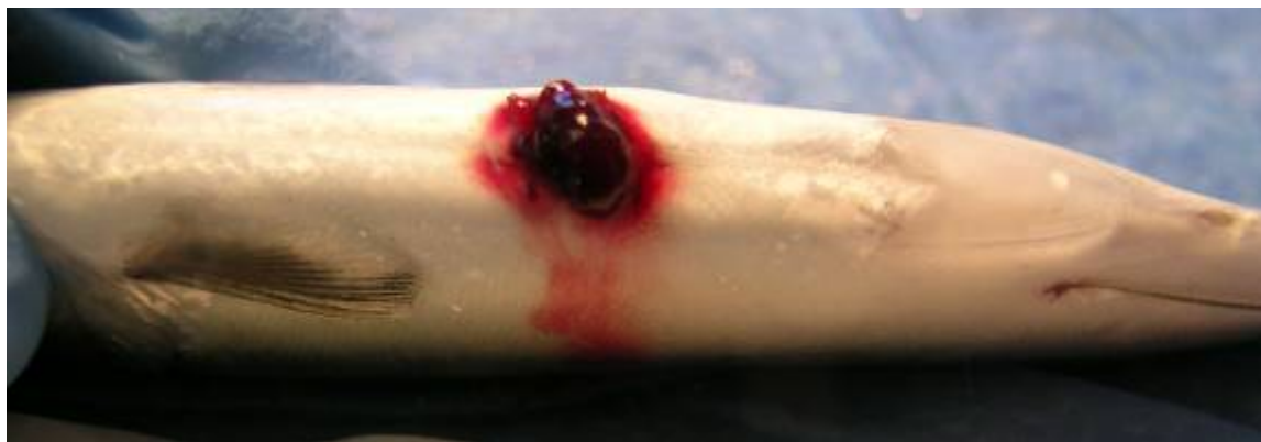
Figure 3.5. Spleen Protruding from the Surgical Incision of a Juvenile Chinook Salmon following Exposure to Simulated Turbine Passage
