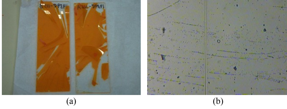
Figure 2.3. Airborne Dust and Organic Compound Contamination. (a) Thin film delamination and (b) thin film particulate contamination.
