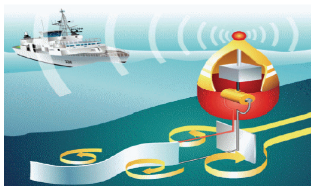
Figure 5.2. Energy harvesting “eel” concept. (Source: Ocean Power Technologies, Inc.)
