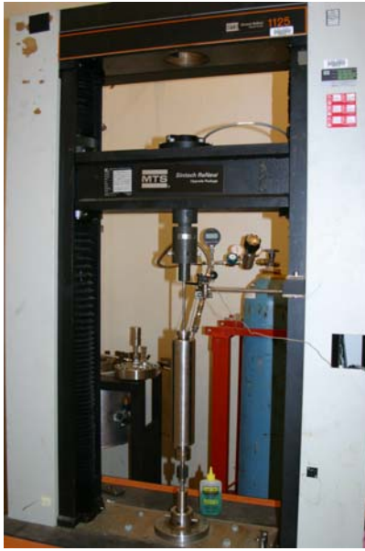
Figure 4: Hydrogen Test Load Frame Set Up and Configuration
