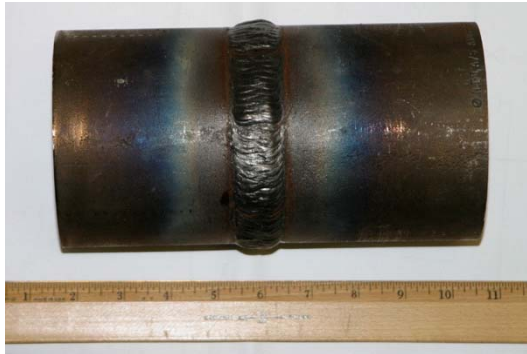
Figure 1: Photograph of Alloy A 106 Grade B Pipe Section after Welding
