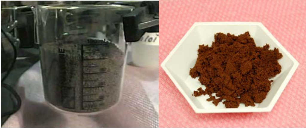
Figure 3-4 Actual Tank 19 Mound Sample Compared to IE-95 Zeolite + Water
