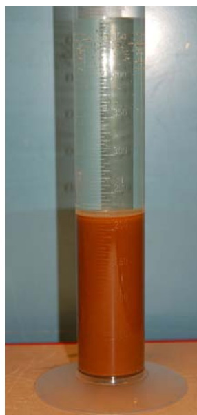
Figure 2-3 Size-Reduced Zeolite in 7 M Na Supernate Settling Test
