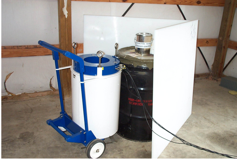
Figure16. Photograph of the Cf-252 activation setup for the AWCC.
