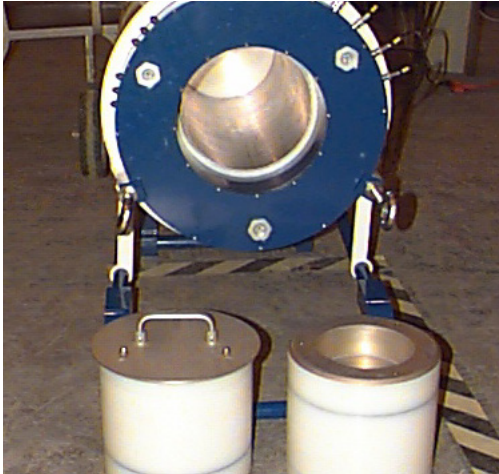
Figure 1. Photograph of SRS K-Area active well coincidence counter lying on its side showing the sample chamber and neutron moderators.
