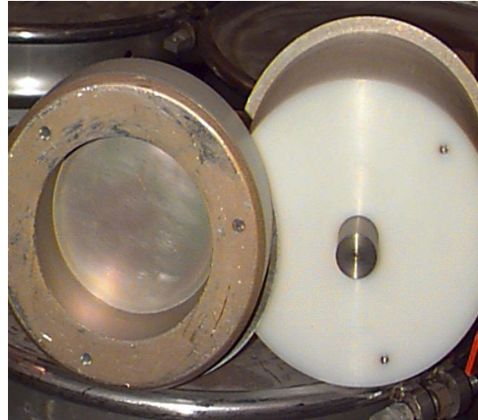
Figure 2. Photograph of one of the Am-Li activation sources and neutron moderator.
