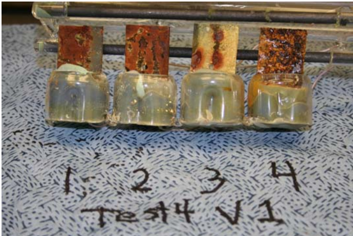
Figure 11. Post-test photo of vertical coupons from Test 4 (50 °C, unmixed). Note goethite and humboldtine on first three coupons.
