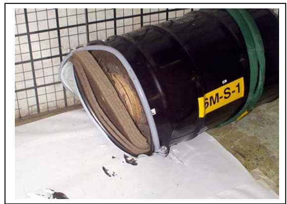
Shallow Angle Drop Damage
