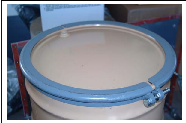
Figure 5 Prototype Clamshell Closure Fitted to a UN1A2 drum
