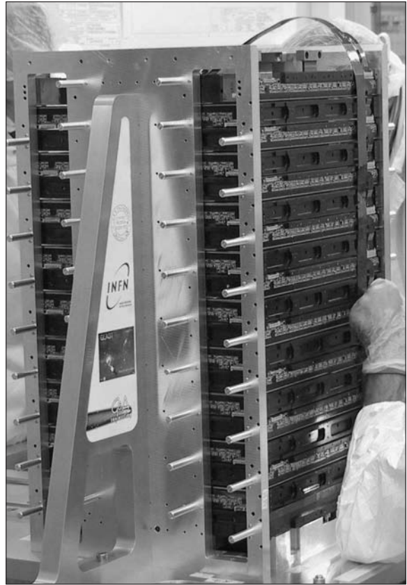
Fig. 9. A tower module being assembled inverted in the precision steel assembly jig, shown during the cable mounting step.
