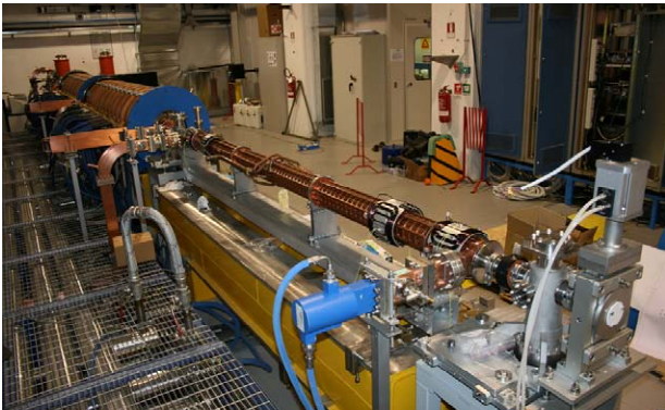
Figure 3: The SPARC linac with the s-band accelerating sections installed.
