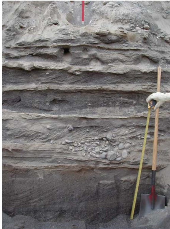
Figure 2.2. Exposed Trench Face Showing Layered Heterogeneity in Hanford's 200 East Area. This trench was located near the south boundary of the ILAW Site.
