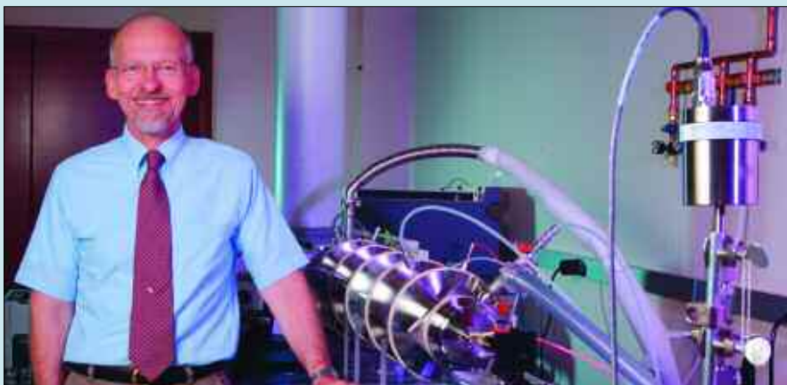
Figure 4. New proteomics platforms can realize even greater potential with the help of FPGAs. Dr. Dick Smith, PNNL, stands with an instrument that incorporates ion-mobility separation with time-of-flight mass spectrometry. The instrument will increase the throughput of proteomics measurements by up to about 100-fold.
