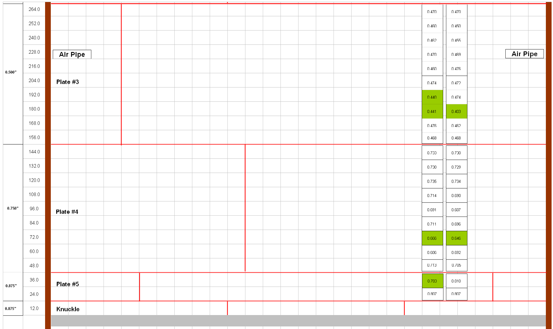
Figure 5.2. UT Data from Tank 241-AY-102 Primary Tank Riser 88 cont.
