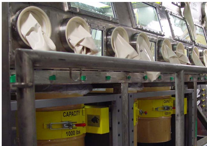
Figure 4. VE glovebox train at a Savannah River Site facility.
