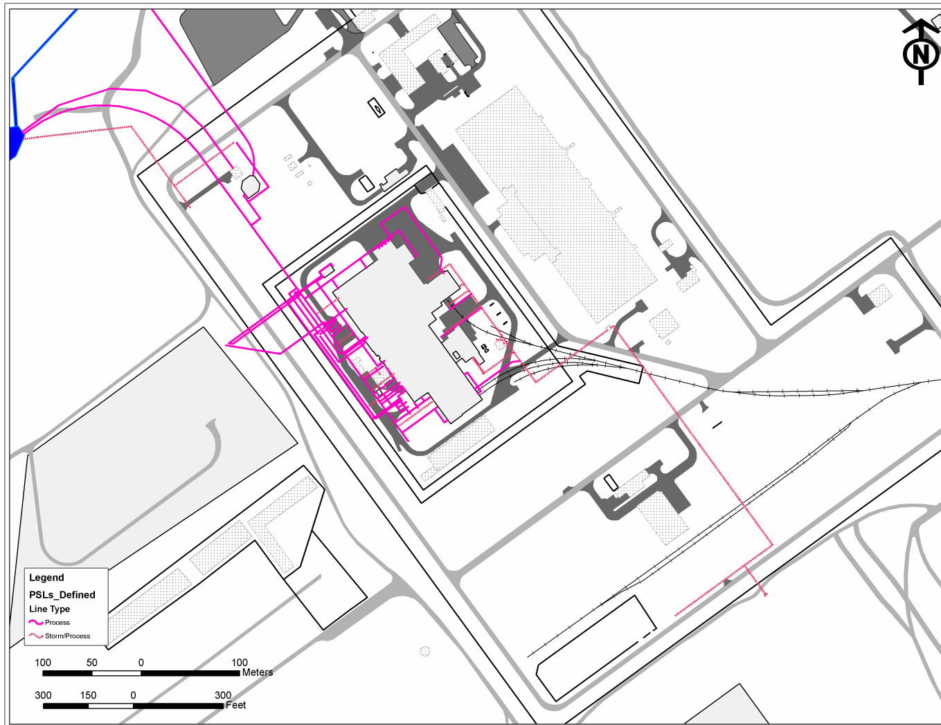
Figure 8: Process Sewer Lines
