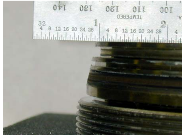
Figure 8. O-ring profile after 1500 hours at 400°F
