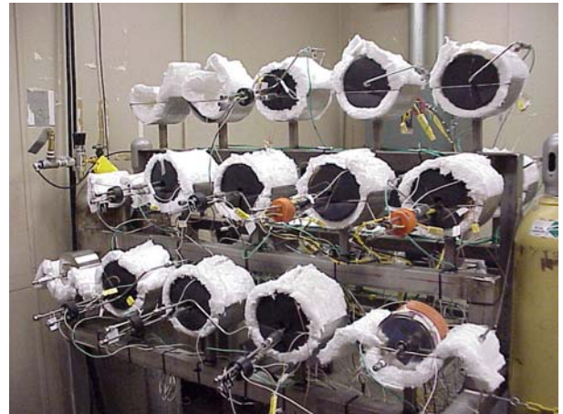
Figure 3. Mock-PCV Storage Rack
