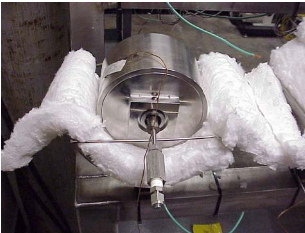
Figure 2. Empty Mock-PCV Fixture Sealed With O-Rings
