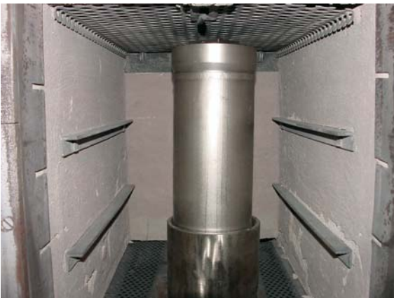
Figure 7. Full-size, empty sealed PCV aged at 400°F
