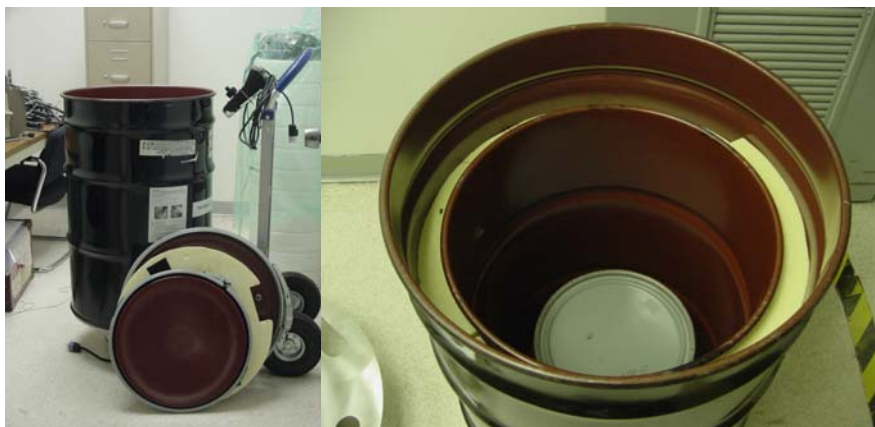
Figure 1. Drum on counting turntable (left) and item in 30-gal/55-gal drum-in-drum configuration.
