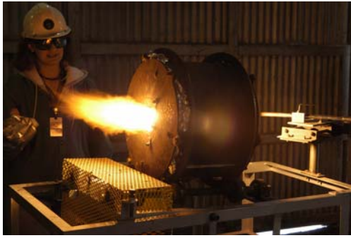
Figure 9: Refractory samples tested for molten slag resistance in the rotary slag test, a) samples during rotary slag testing, and b) non-chrome and chrome based refractories after rotary slag testing. Testing was for 4 hours of exposure to a coal gasifier slag at 1667°C.
