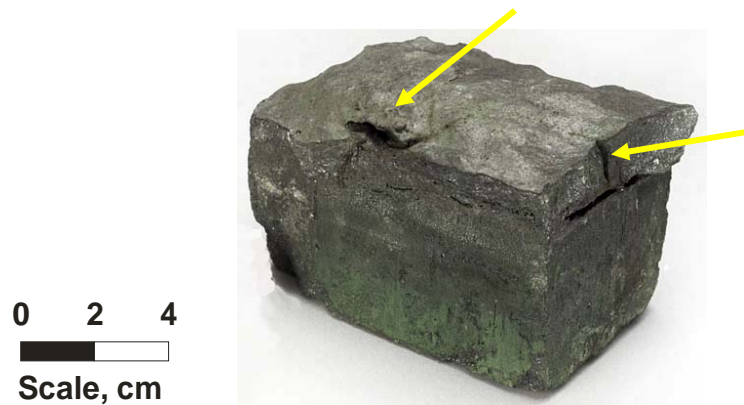
Figure 2: Examples of refractory wear caused by slag dissolution and spalling: a) Flowing slag is causing chemical dissolution of the refractory sidewall and refractory material spalling (circled fragment). b) Thin spalled refractory shown fig 2 (a). c). Thick spalled refractory.
